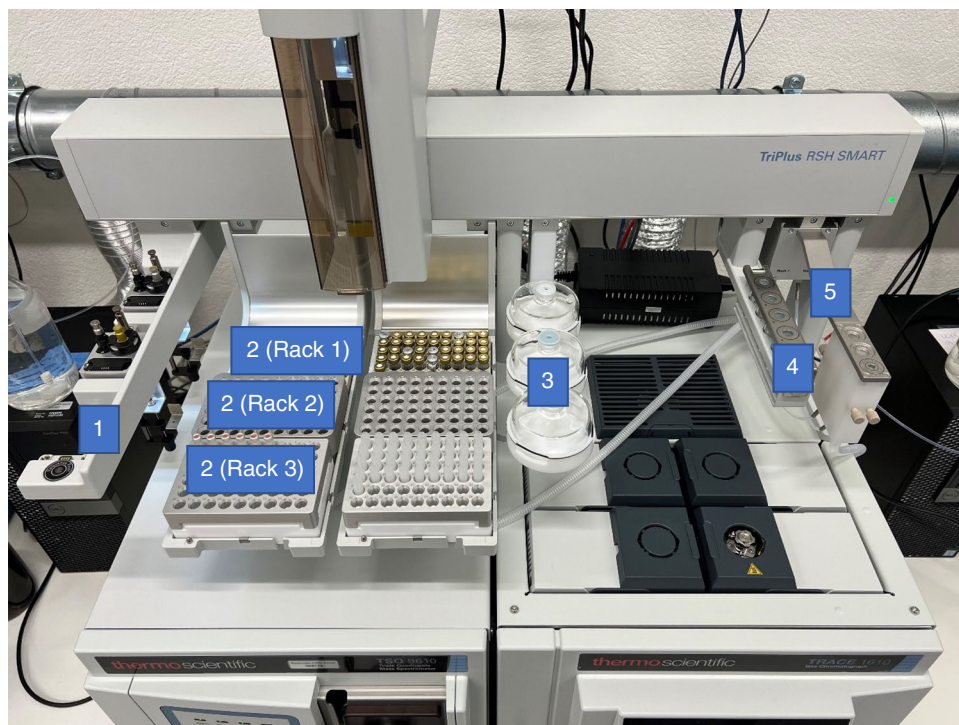
Fig. 1 TriPlus RSH SMART system configuration for automated \mu SPE extract clean-up. 1, automatic tool change (ATC) station with 10-, 25-, and 1000- \mu L syringes; 2, \mu SPE tray with rack for raw extracts in 2-mL vials, elution rack into 2-mL vials, and \mu SPE cartridge rack; 3, solvent module for 3 \times 100 mL reservoirs for solvents; 4, standard wash station for location of standards and APIs in 2-mL vials; 5, fast wash station for syringe cleaning
